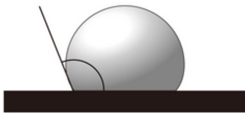
Fig.1 Hydrophobicity (contact angle is large)
