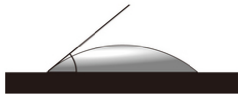
Fig.2 Hydrophilicity (contact angle is small)
